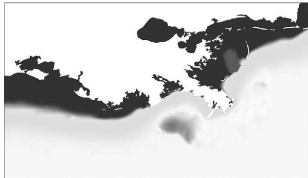
Fig. 19. Flooding near the Louisiana coast, T \approx 10 h (gray shading indicates elevation above original water surface).
