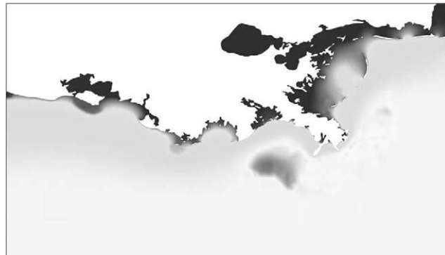
Fig. 20. Flooding near the Louisiana coast, T \approx 33 h (gray shading indicates elevation above original water surface).
