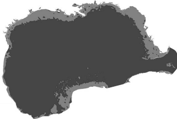
Fig. 16. Initial bathymetry and coastal elevation (black indicates initial water surface; gray indicates dry areas).
